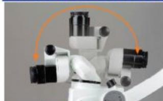
0° - 180° inclinable binocular tube
