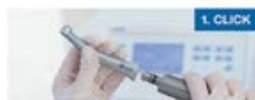
Attach the contra-angle to the motor so that it snaps into place.
